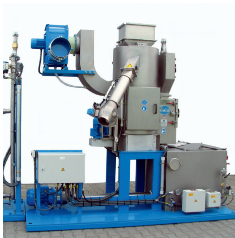
TWS-20 with IS water tank and 2016BF Dryer
